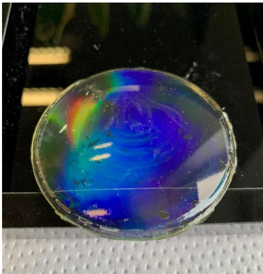
Figure 3. AR-Moth-Eye structure demonstrated on a 3D printed lens. The front and backside of the lens is imprinted with AR-Moth Eyes. The homogeneous imprint and coverage is shown by illuminating at a very flat angle of incidence.
