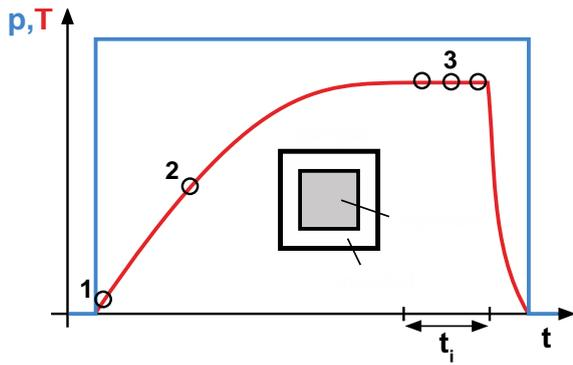
Figure 1. Typical imprint procedure used for PHP of  $\text{MAPbBr}_3$  –  $p = 100$  bar,  $T_i = 150^\circ\text{C}$ ,  $t_i = 5$  min, heat-up time 20 min. The labels refer to specific situations characterized in Fig. 2 – 4.
