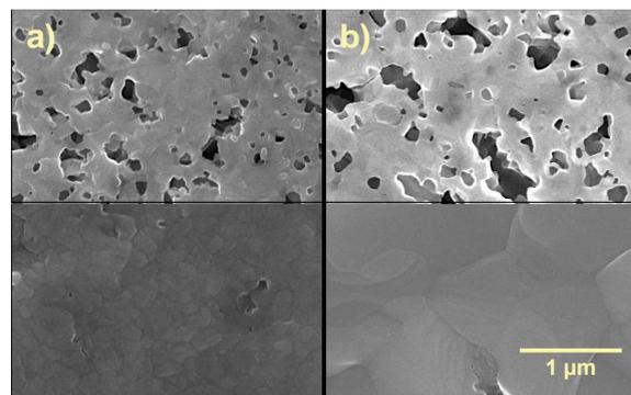
Figure 6. Pure annealing experiment –  $75^\circ\text{C}$  (top) /  $125^\circ\text{C}$  (bottom); a) 1 min, b) 20 min. (nitrogen atmosphere)
