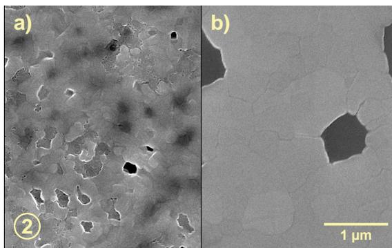
Figure 3. Simulation of the impact of a reduced temperature – a) annealed part, b) imprinted part (HL, 100 bar,  $75^\circ\text{C}$ , 60 min).
