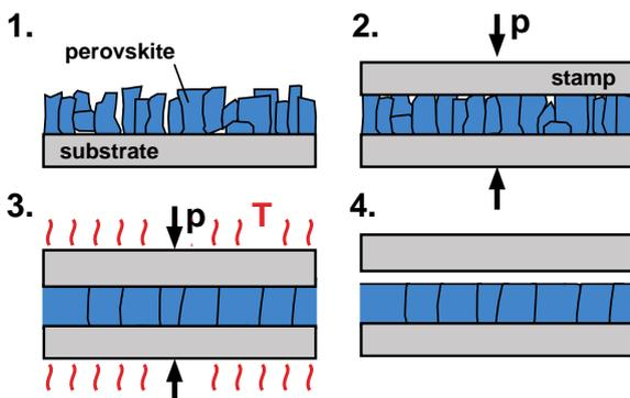
Figure 5. Perception developed from the simulation experiments – 1. Pristine layer, 2. compression, 3. grain growth, 4. final layer
