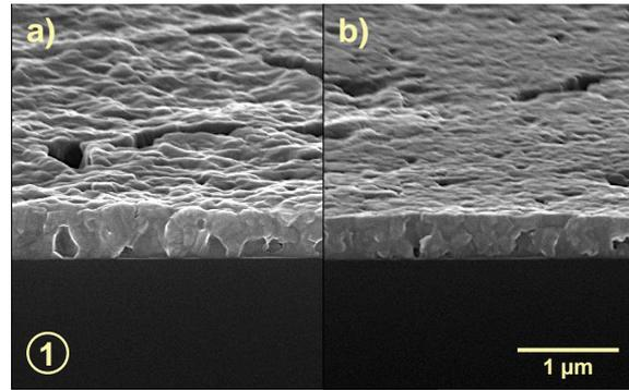
Figure 2. Simulation of the impact of pressure – a) annealed part, b) imprinted part (HL, 100 bar, RT, 60 min).
