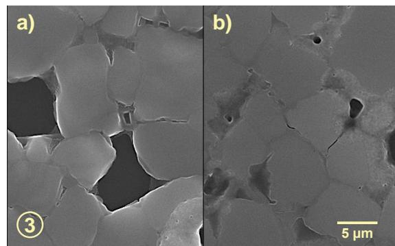
Figure 4. Simulation of the impact of a typical imprint temperature – a) annealed part, b) imprinted part (HL, 100 bar,  $150^\circ\text{C}$ , 5 min).
