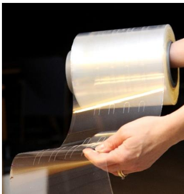
Figure 1 Roll of R2R imprinted \mu fluidic channels in PDMS. Web width 200mm.
