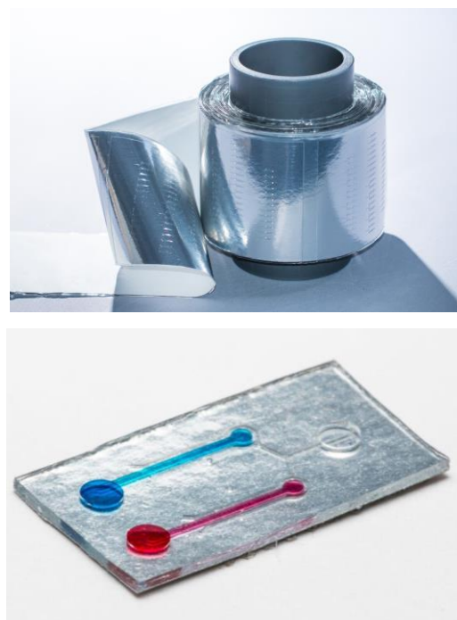
Figure 2 a) Roll of replicated PDMS fluidics on aluminized paper in width of 100mm. b) RNA amplification device filled with blue and red color [2]
