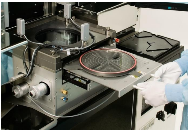
Figure 2. Mask aligner (Suss MicroTec) for imprint lithography and wafer stacking
