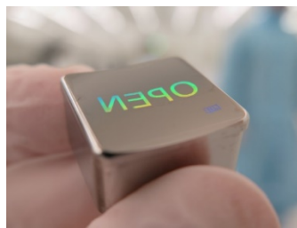
Figure 6: Digital camera image of curved steel insert with diffractive structures.
