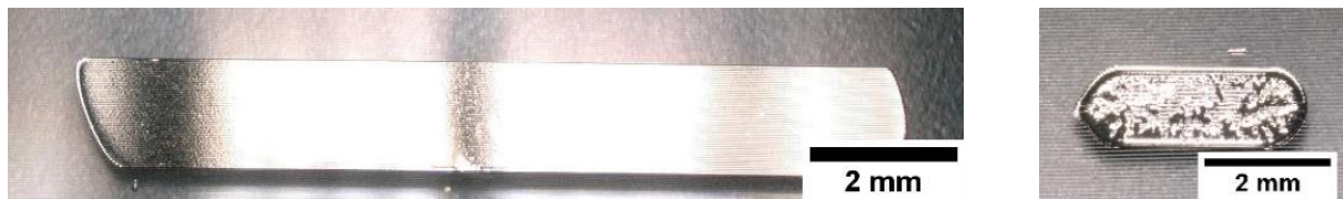
Figure 3. Microscope image V-grooves of 31\ \mu\text{m} periodicity imprinted in OrmoComp (micro resist technology) with nanoparticle inks (PV Nano Cell) manually deposited on top. The left image shows the resulting conductive lines for an ink that has a low contact angle \theta fulfilling the capillary filling condition \theta < (\pi - \alpha)/2 [4]. The original deposited droplet vanishes completely and fills the microchannels up to a length of 1 cm. Right: A nanoparticle ink with a higher contact angle deposited on the same structure stays within the deposited region.
